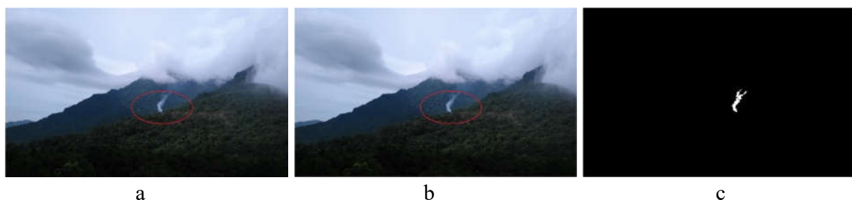
Figure 2. Day-time smoke test block; (a, b) consecutive frames; (c) Image after processing
