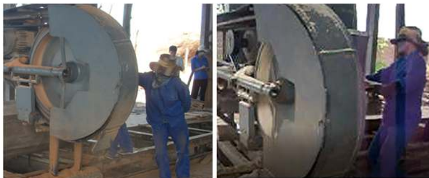
Figure 2. Push and pull operation when operating the HLBS machine
