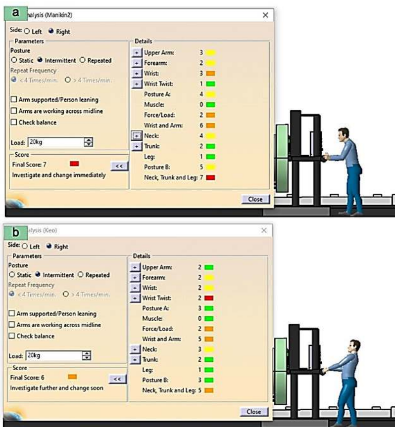
Figure 8. RULA score of 95th percentile worker during pushing (a) and pulling (b) operation
